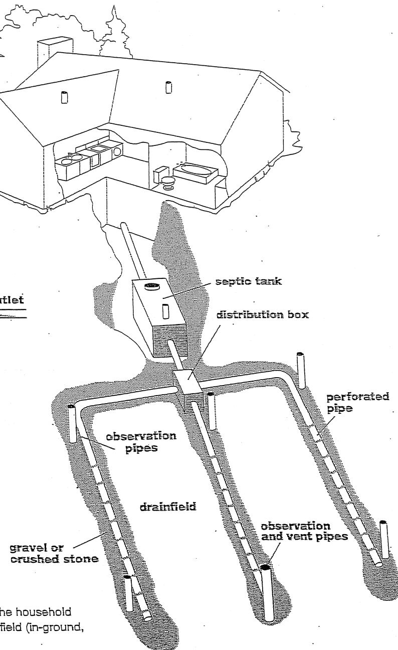
Residential septic systems include the household plumbing, a septic tank, and a drainfield (in-ground, at-grade, mound, or seepage pit).
